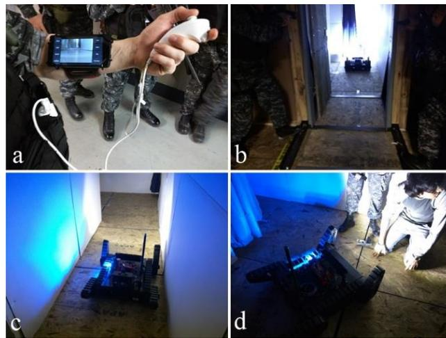
**Fig. 4.** Use of current interface in SWAT training a) team member with the interface b) robot entering the apartment, c) robot checking the hallway with activated strobe and sound, and d) robot assists in capturing the suspected threat.
