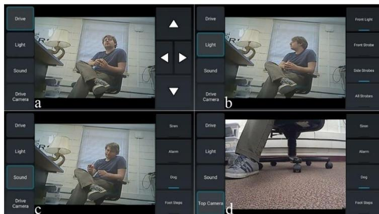
**Fig. 3.** Current Iteration – camera broadcast always visible: a) drive controls, b) lights and strobes options, c) diversion sounds options, and d) toggled camera showing drive camera
