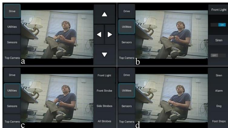
**Fig. 2.** Second Interface Iteration – camera broadcast always visible: a) drive controls, b) light and sound control as utilities, c) lights and strobes options, and d) diversion sounds options.
