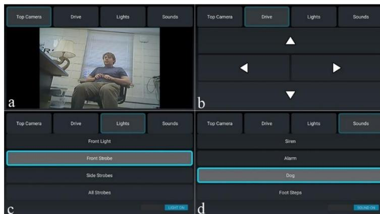
**Fig. 1.** First Interface Iteration: a) broadcast panel from top camera, b) drive controls panel, c) lights and strobes options panel, and d) diversion sound options panel.
