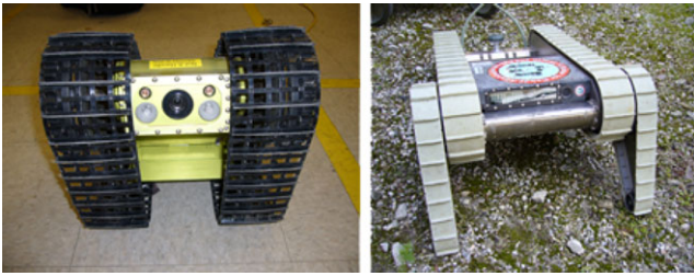
Fig. 2 The Robots: Inuktun Extreme-VGTV (left) and iRobot Packbot Scout (right)
