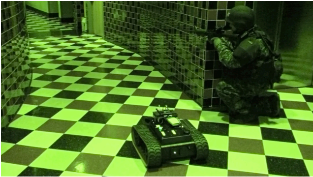
Figure 2: MMP-30 robot from the Machine Lab customized by Clearpath Robotics, Inc.
